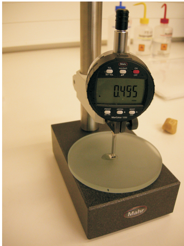
Figure 6.3: Thickness measurement of die with thickness of 495 \mu\text{m} , mounted on a rigid glass carrier, by means of a digital measurement unit
