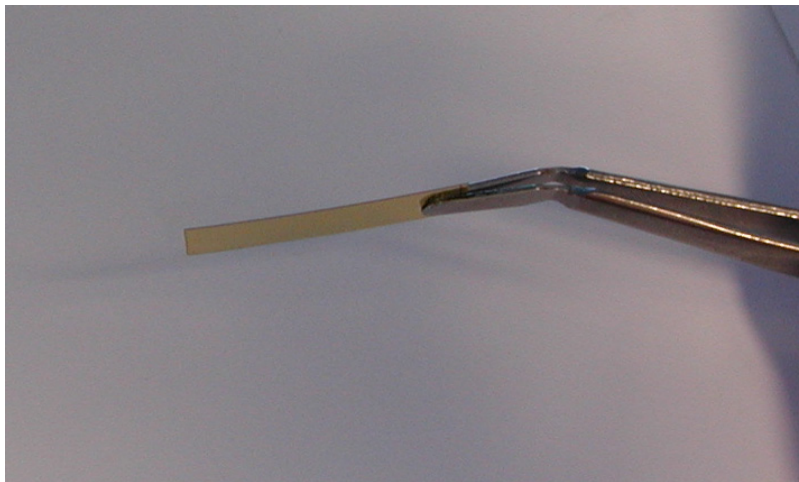
Figure 5.6: Flatness of sandwich of 5 μm PI-2611/30 μm HD-7012/5 μm PI-2611 after release from rigid carrier
