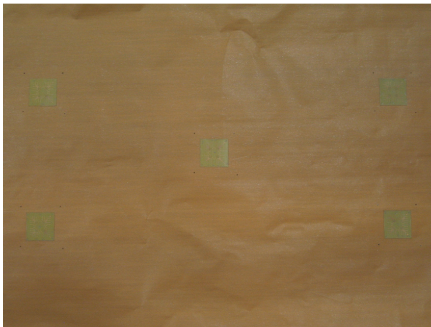
Figure 4.3: Placement of 5 small, 2 \times 2 \text{ cm}^2 , UTCP dummy packages all over the large commercial ACB flex sheets (panel size: 305 \times 457 \text{ mm}^2 )
