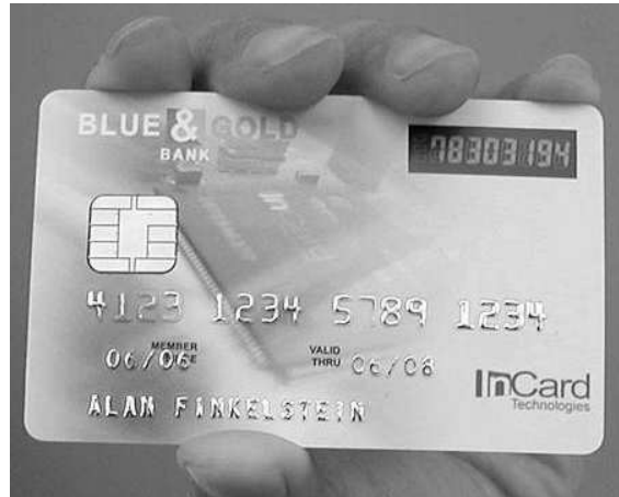
Figure 4.16: Smartcard with a bistable display
