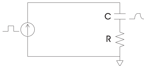
Figure 8.2: Circuit to measure the display capacitance
