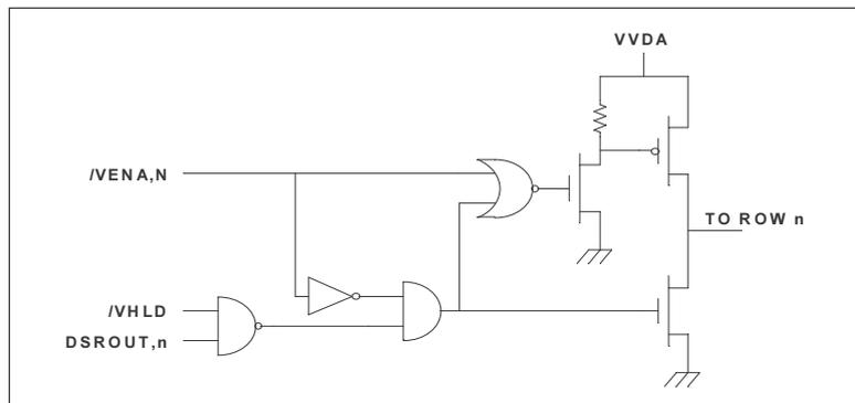
Figure 6-35 : row driver enable logic
