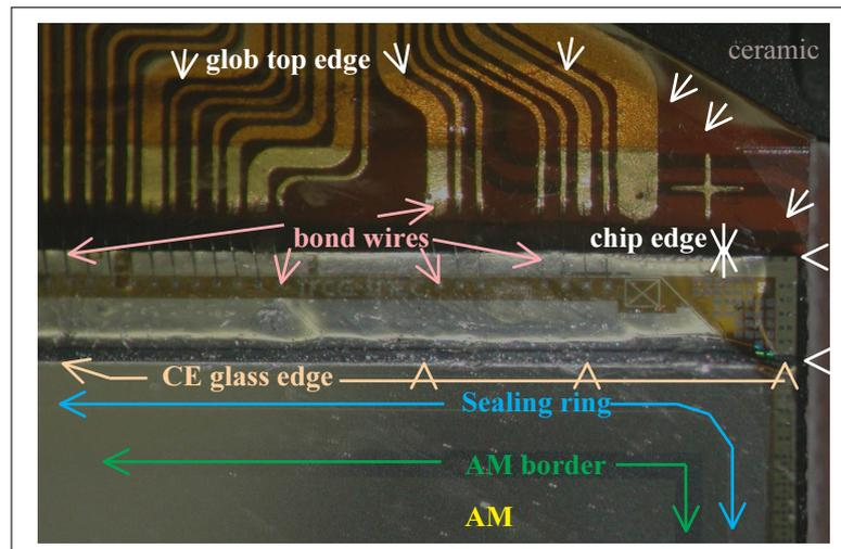
Figure 2-19 : XGA wire bonding to flex substrate with 'glob top' protection
