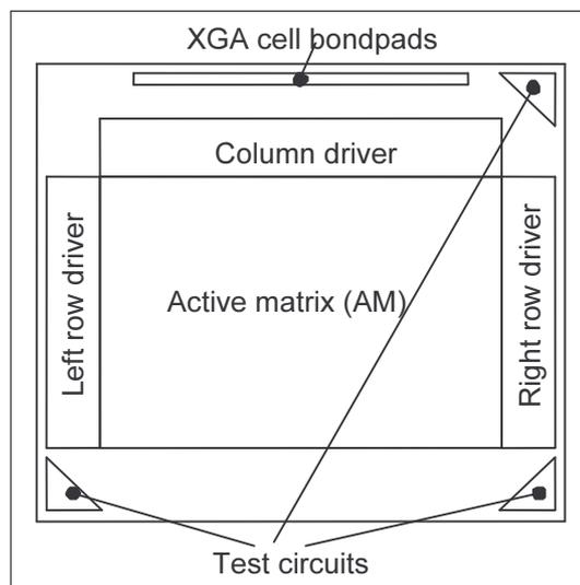
Figure 6-46 : tmdc XGA block diagram
