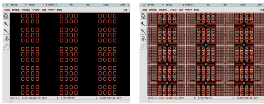
[a] nwell mask, source/drains of trits] [b)with active area and poly masks]
