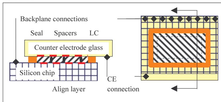
**Figure 1-11: a first glance at an lcos micro-display**
