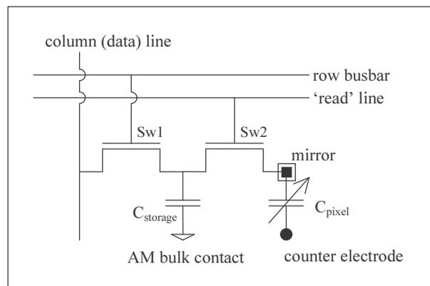
Figure 5-9: two-transistor pixel circuit
