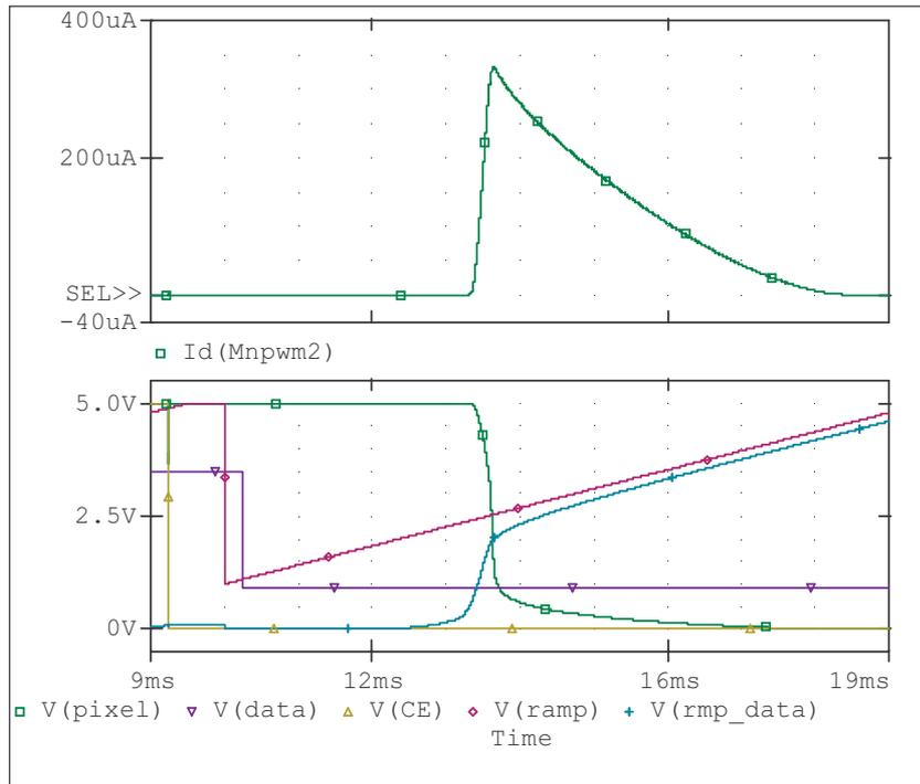
**Figure 5-17: basic PWM operation – transition current**
