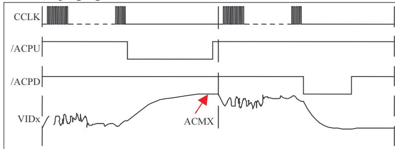
**Figure 6-51 : active clamping signals**
