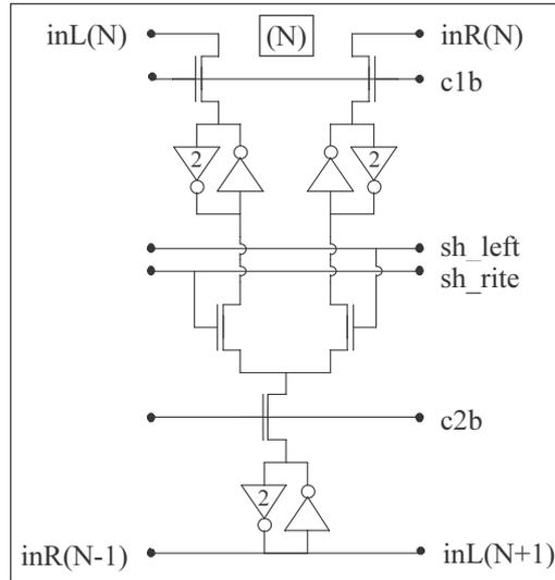
**Figure 6-12 : 160x120 bidirectional scanner element**
