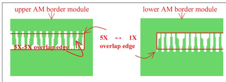
**Figure 3-6 : correction for 1X-5X and 5X-5X positioning errors; the two modules serve as link between the 5X active matrix and the 1X periphery**
