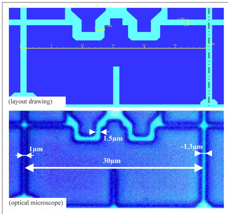
**Figure 3-18 : a microscope picture of developed photo-resist shows the clearly noticeable effect of double exposures**
