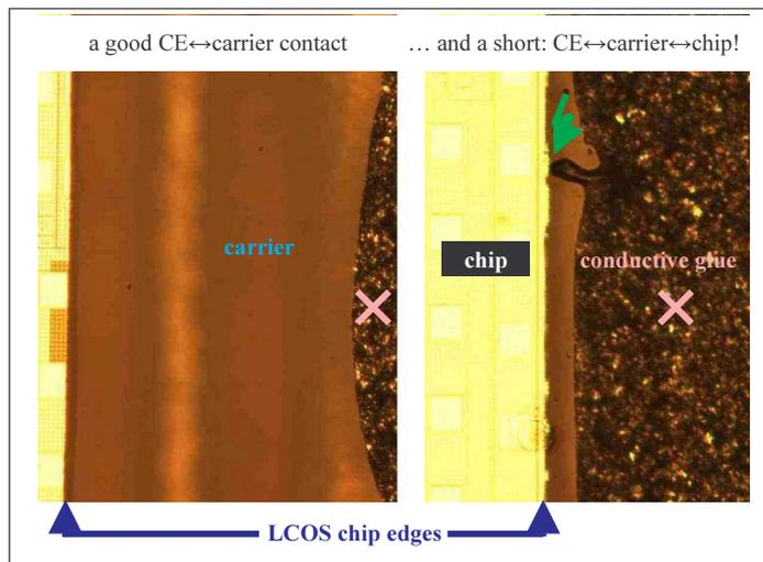
Figure 2-21 : examples of a good (left) and bad (right) CE contact directly between the carrier and the CE
