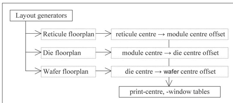
Figure 3-21 : stitching procedure output data for the stepper-job
