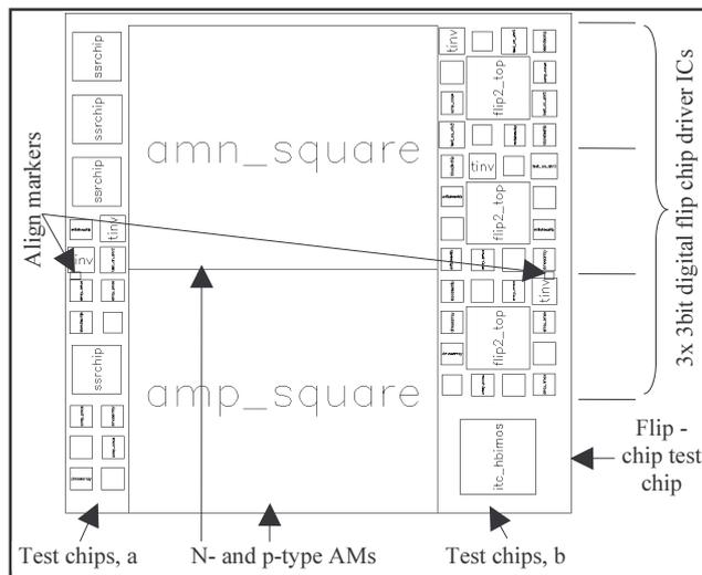
Figure 6-7: quarter-wafer floorplan
