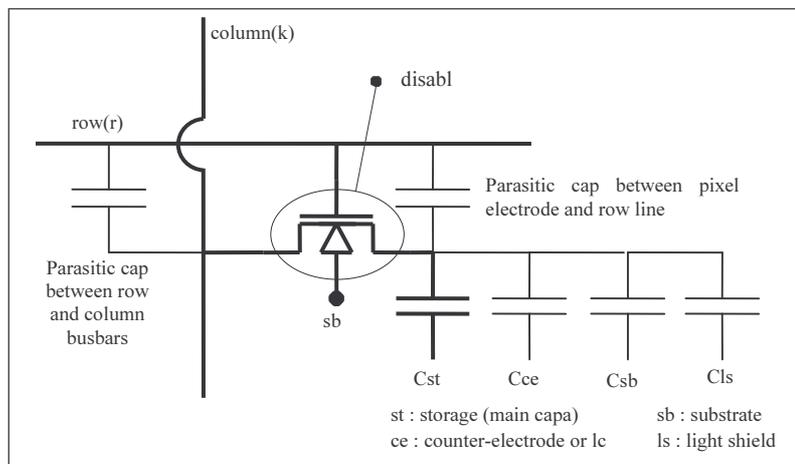
**Figure 6-52 : pixel schematic**
