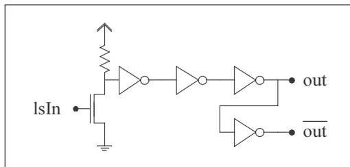
**Figure 6-13 : 5 to 15V level shifter schematic**
