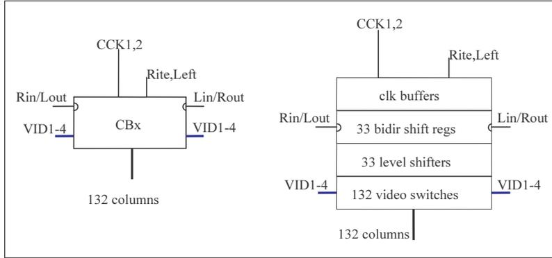
**Figure 6-53 : block schematic of one ‘CBx’**
