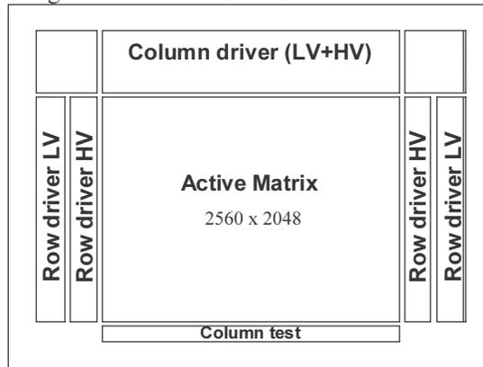
**Figure 6-31 : GXGA block schematic**
