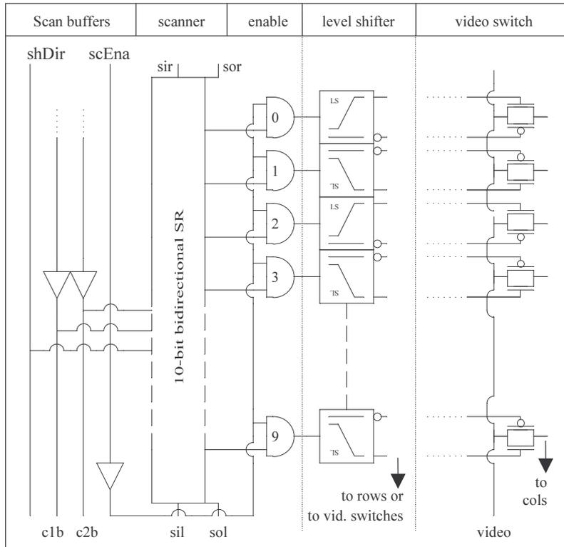
**Figure 6-11 : 160x120 row and column driver building block**
