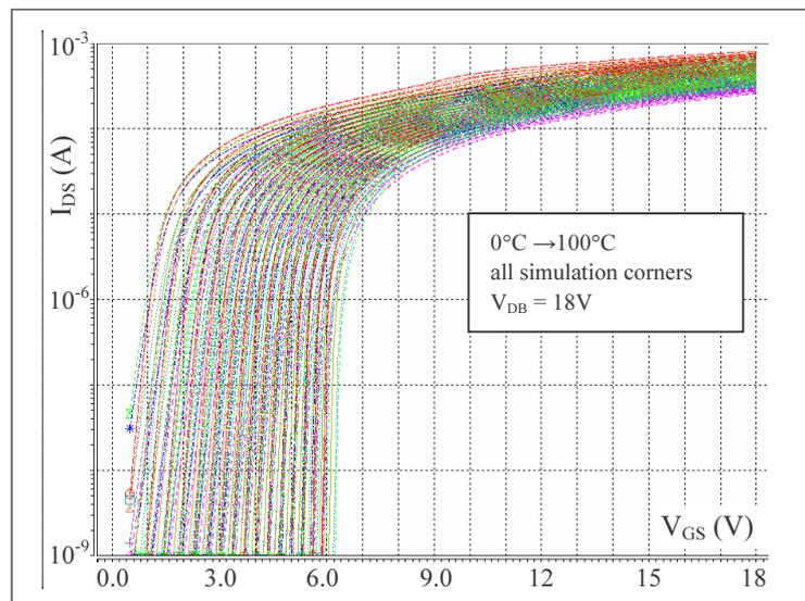
**Figure 4-4: bulk effect simulation for a 3 $\mu$  NMOS**
