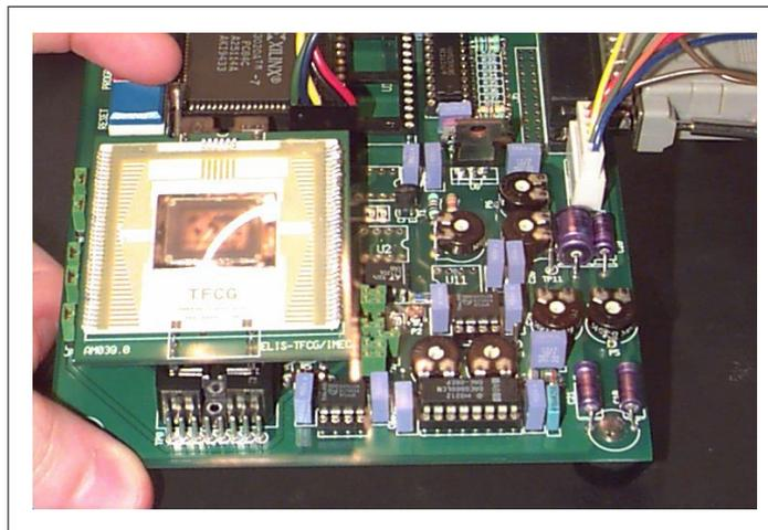
Figure 2-17 : 120x160 wire bonded to plated substrate
