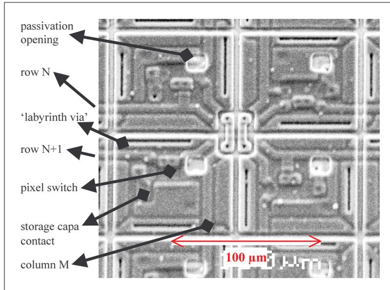
**Figure 4-12: 'reflec' pixel quad seen by a SEM**
