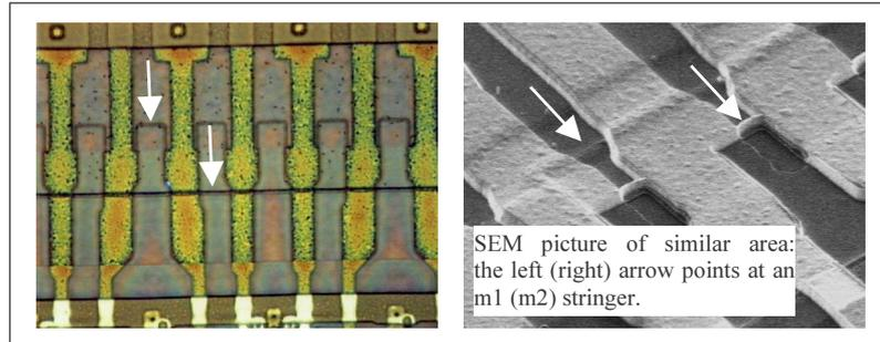
**Figure 3-11 : stringers along the edges of the stitching overlap area**
