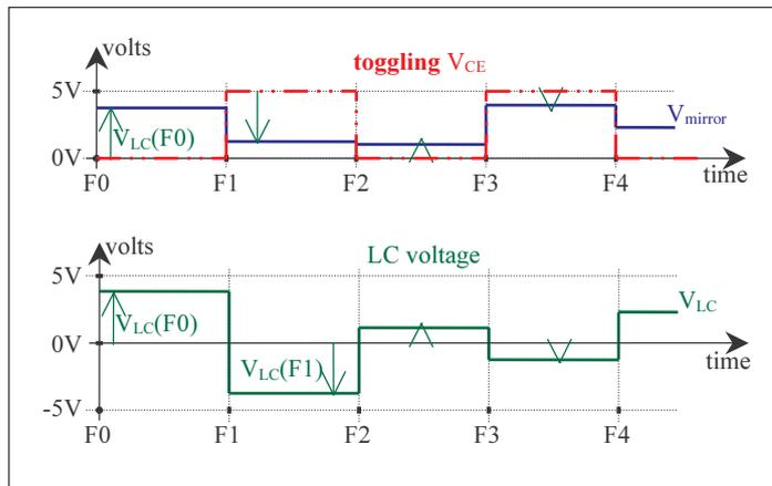
**Figure 5-3: identical LC voltage obtained with CE switching**
