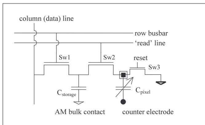
**Figure 5-11: reset transistor to cancel the image retention issue**
