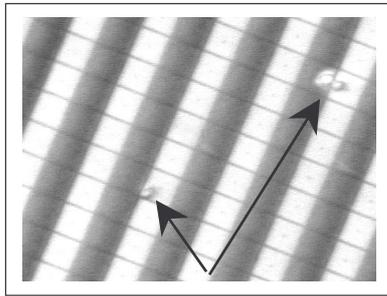
**Figure 2-11 : spacers on 15µm VAN pixels**
