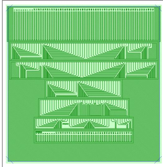
**Figure 6-15 : second nwell and metal2 reticles**
