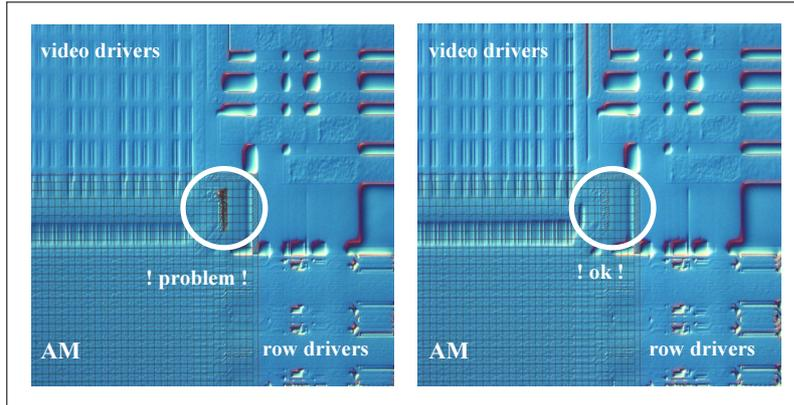
**Figure 3-13: chips with (left) and without (right) planarity problems**
