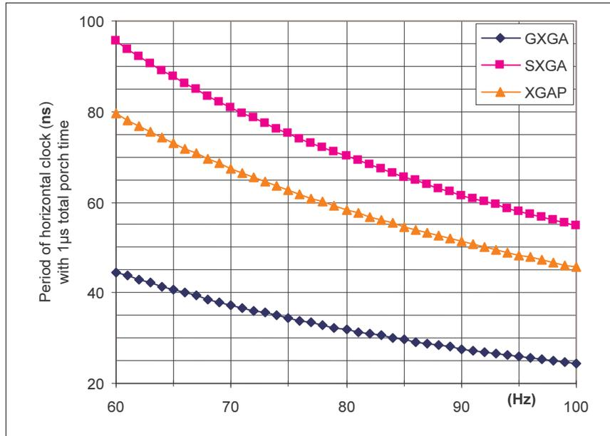
**Figure 6-25: HCLK period as function of the frame rate**
