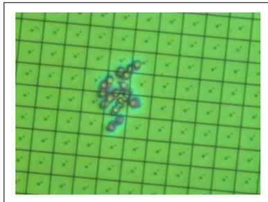
**Figure 2-12 : an undesirable cluster of spacers in a MOSAREL cell**
