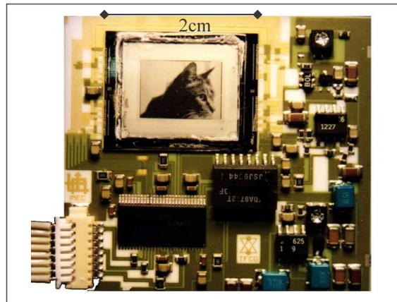
**Figure 2-7 : 160x120 80 $\mu$  PDLC panel**
