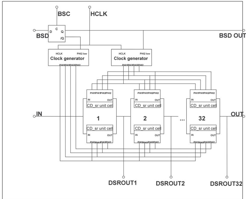
**Figure 6-37 : column driver shift register sub-block**
