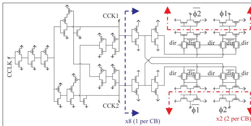
**Figure 6-55 : column-clock buffer tree**
