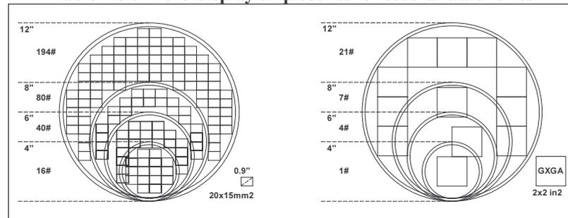
Figure 2-25: relative wafer sizes and corresponding chip counts
