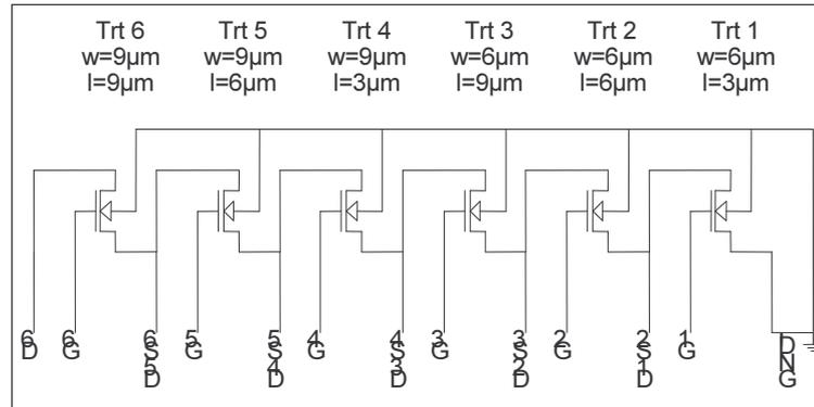
Figure 6-5 : SiLCD test transistors schematic
