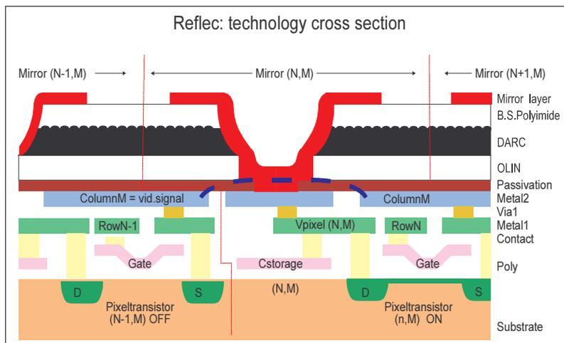
**Figure 4-9: schematic 'reflec' backplane cross section**
