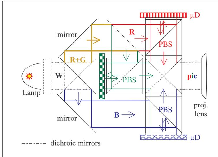
**Figure 1-7: three-panel reflective architecture**
