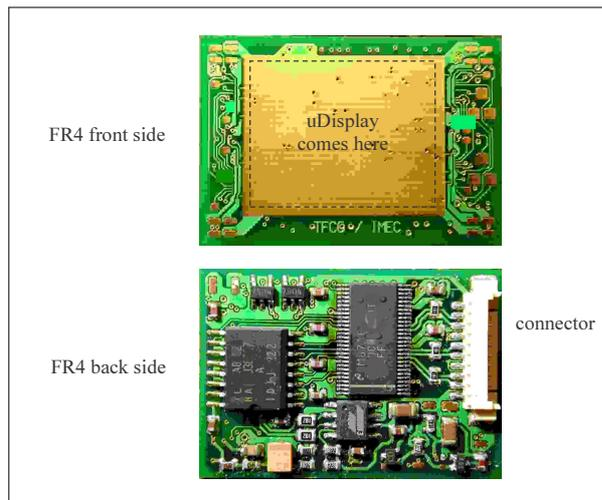
Figure 4-15: 'reflec' demonstrator with components on the back of the carrier
