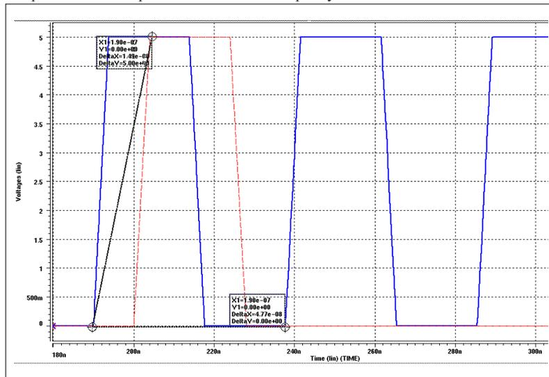
**Figure 6-28 : GXGA column-driver timing data**
