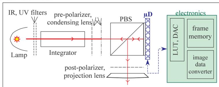
**Figure 1-5 : a basic monochrome lcos setup**
