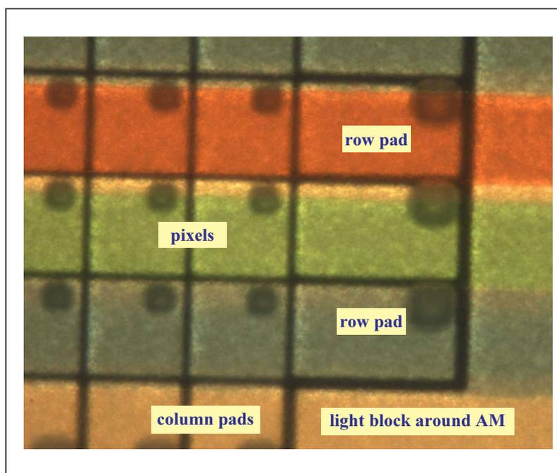
**Figure 4-10: a 'reflec' chip with colored pixels**
