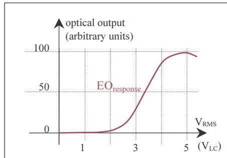
**Figure 4-1: the electro-optical response as function of RMS voltage**
