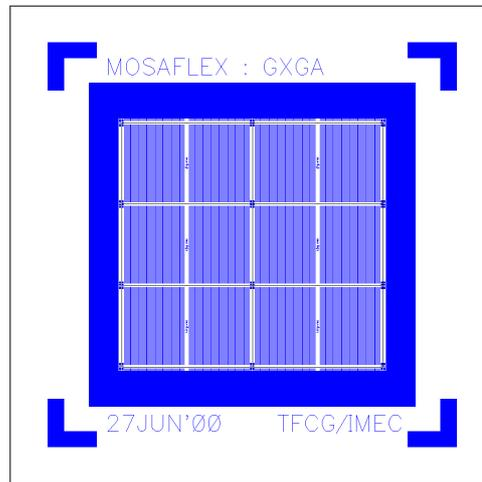
Figure 2-18 : mask for 6 128-pin flexes, see also Figure 2-8
