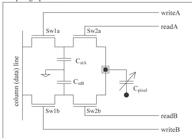
Figure 5-14: the double dram circuit
