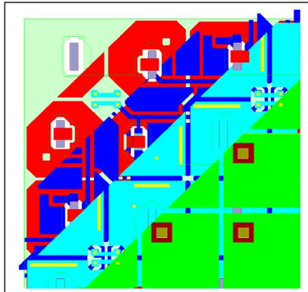
**Figure 2-6 : layout (or top-) view of a Si backplane (3x3 pixels approximately)**
