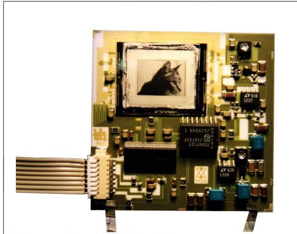
Figure 4-14: 'reflec' on a ceramic carrier with SMD components
