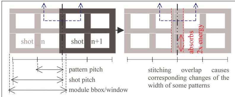
**Figure 3-17 : top view of an area exposed two times**
