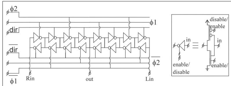
**Figure 6-58 : a bidirectional shift-register element**
