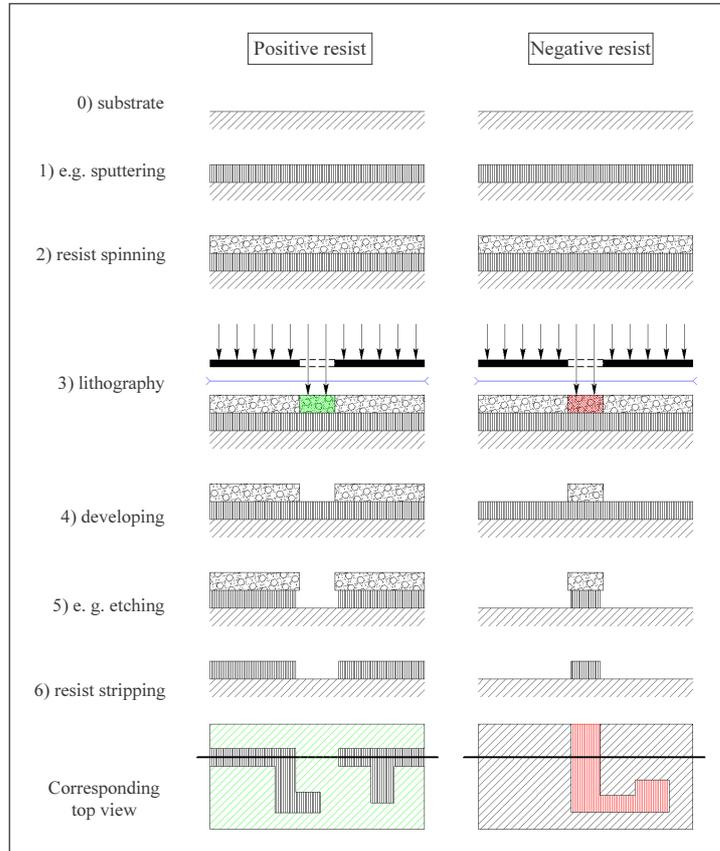
**Figure 2-24 : lithography with positive or negative resist**
