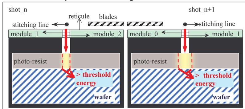
**Figure 3-16 : cross section view of an area exposed two times**
