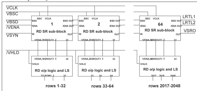
**Figure 6-43 : row driver with 2048 outputs**
