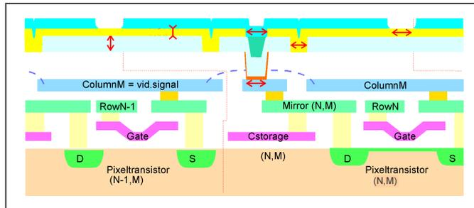
**Figure 2-5 : Si backplane cross section**
