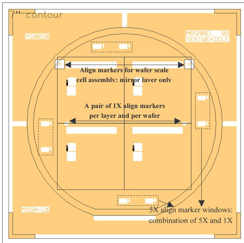
Figure 2-26 : picture of a 1X mirror layer mask (6" wafers)
