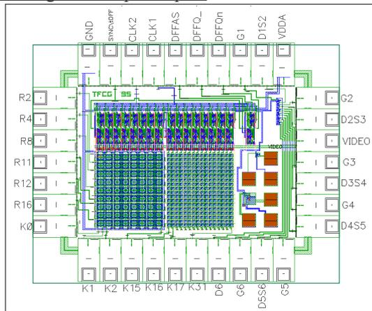
**Figure 6-1 : SiLCD chip layout**
