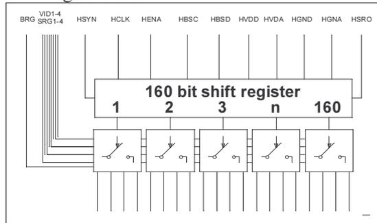
**Figure 6-32 : schematic of column driver segment**
