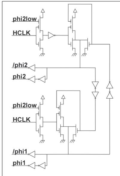
**Figure 6-39 : clock generator circuit**
