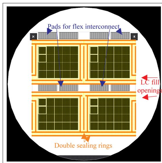
**Figure 2-16 : MOSAREL double sealing ring design**
