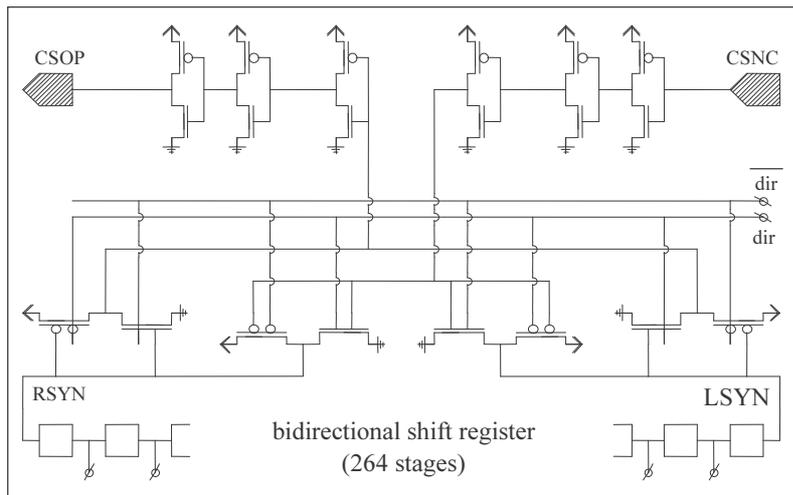
**Figure 6-57 : sync-in and -out plus buffers**
