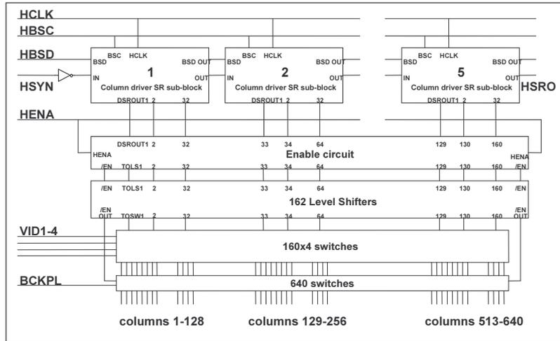
**Figure 6-36 : 640 o/p column driver segment block schematic**
