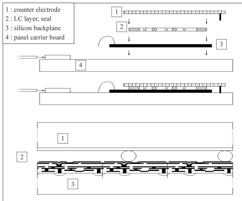
Figure 2-4 : cell cross section
