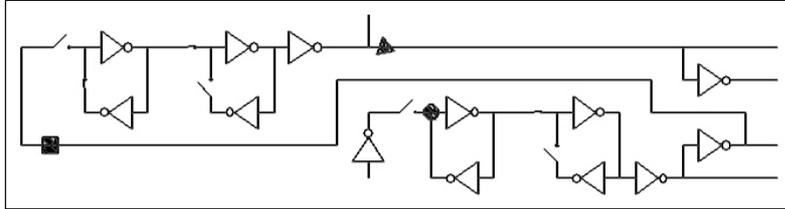
**Figure 6-4 : 2-stage shift register schematic**
