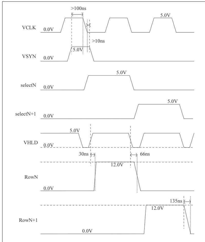
**Figure 6-26 : GXGA row-driver timing data (part 1)**
