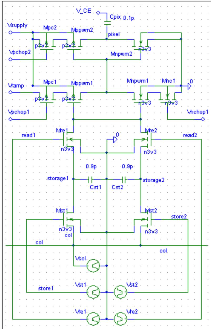
Figure 5-18: spsice circuit of the combination of a double dram pixel memory block, plus a smart current-limited PWM circuit block
