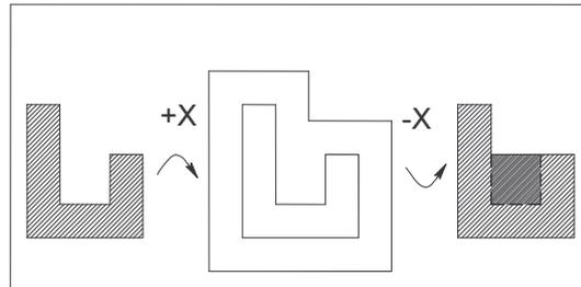
Figure 6-77 : +x, -x fills narrow 'notches', ok
