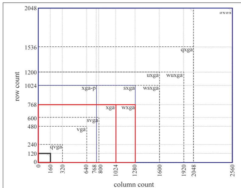
Figure 4-7: image format comparison at constant pixel pitch
