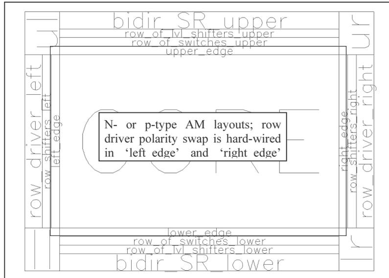
**Figure 6-8 : 160x120 backplane chip floorplan**
