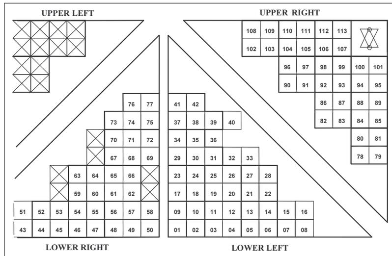
**Figure 6-64 : corner floorplan and numbered probe pad configuration**
