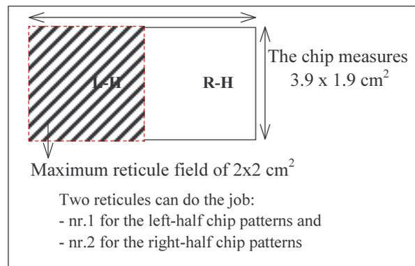
**Figure 3-1: two reticules for one masking step**
