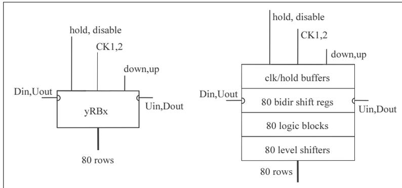
**Figure 6-60 : block schematic of the row blocks**
