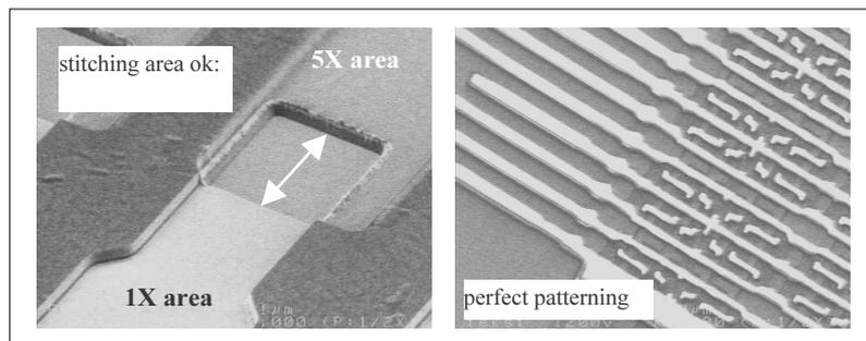
**Figure 3-12 : corrected processing for a perfect result**
