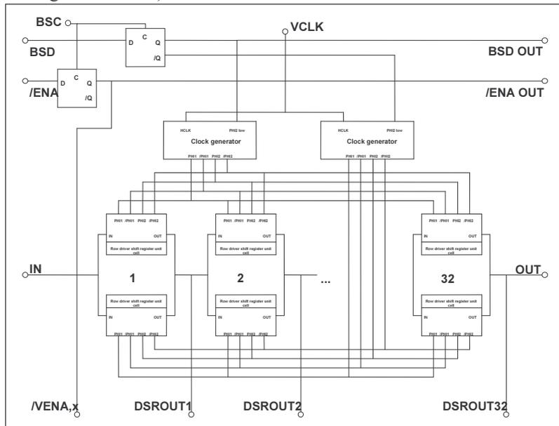
Figure 6-44 : row driver shift register sub-block
