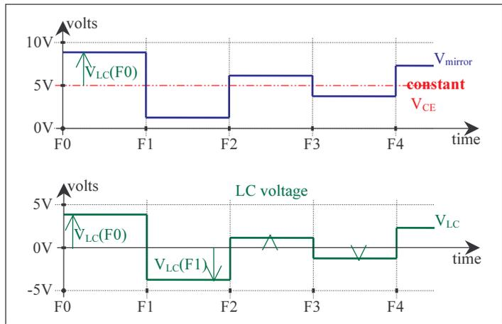
**Figure 4-5:**  $V_{mirror}$  with respect to chip ground and resulting  $V_{LC}$
