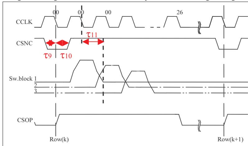
**Figure 6-50 : column driver signals**
