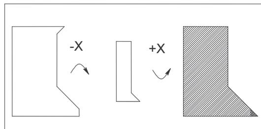
Figure 6-80 : -x, +x results in 'overgrow'; solved by 'anding' with the source
