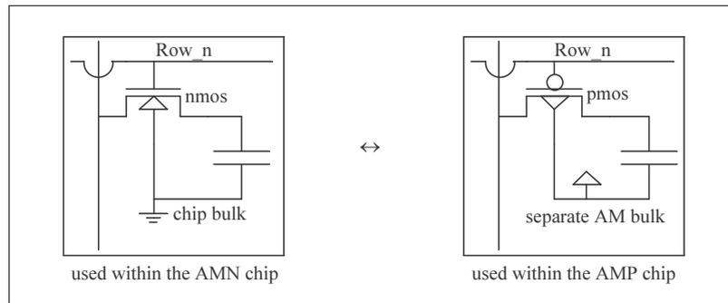
**Figure 6-10 : two 'REFLEC' pixel architectures**
