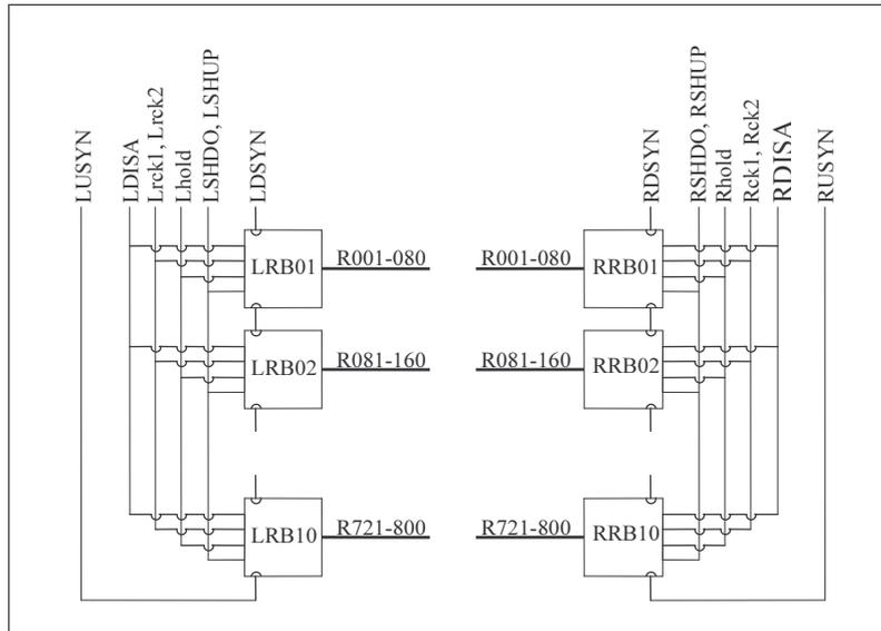
**Figure 6-62b : block schematic of the (double) row driver**
