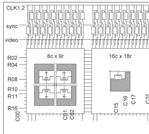
**Figure 6-3 : SiLCD main circuit schematic**
