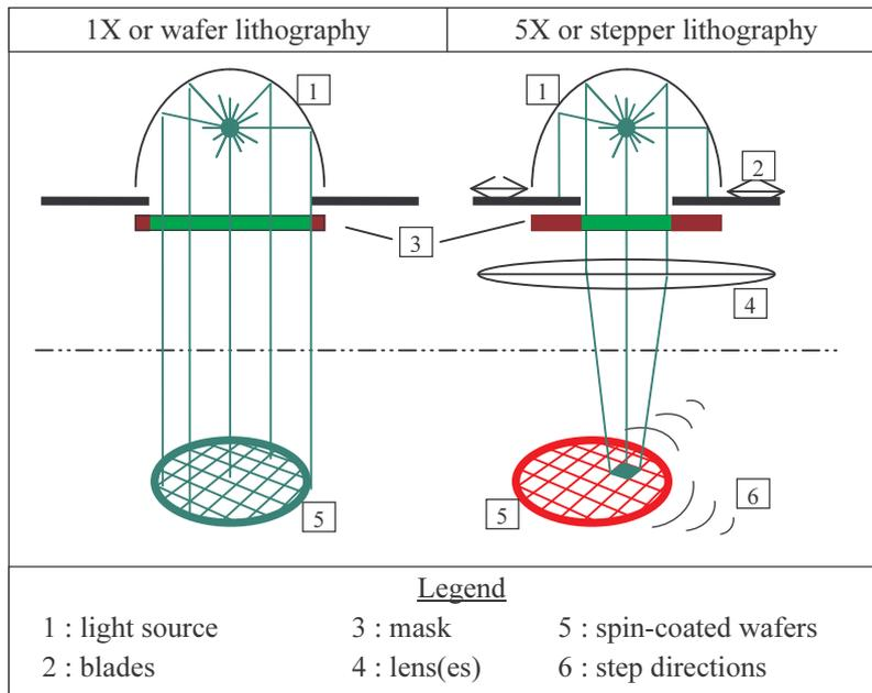
**Figure 2-28 : contact printing and stepper mechanisms**
