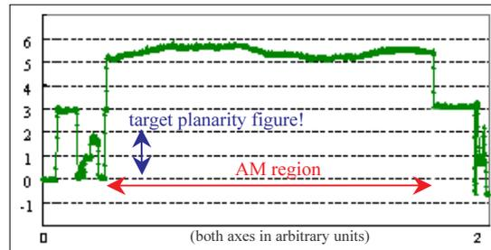
**Figure 2-14 : typical  $\mu$ display chip topography prior to the metal (aluminum) depositions**
