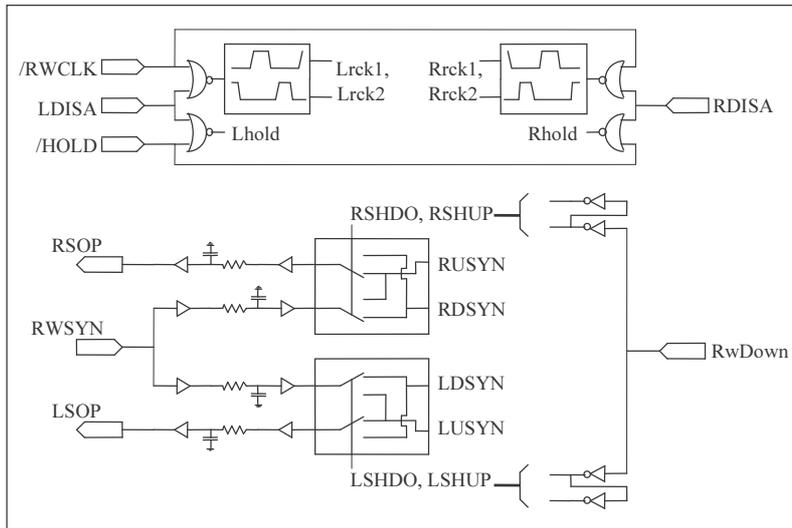
**Figure 6-61a : block schematic of the (double) row driver**
