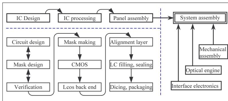
**Figure 2-2 : lcos manufacturing chain(s)**
