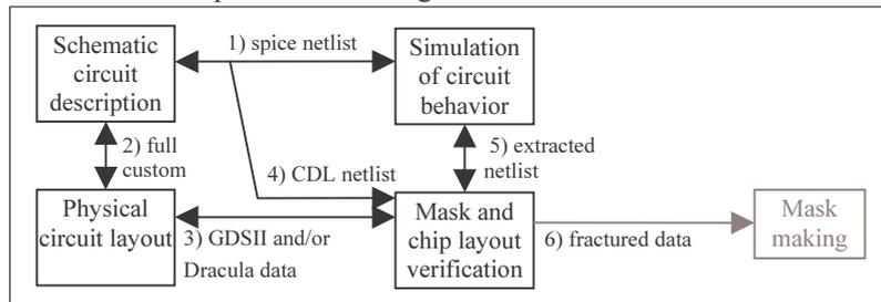
Figure 2-3: an (lcos) IC design cycle
