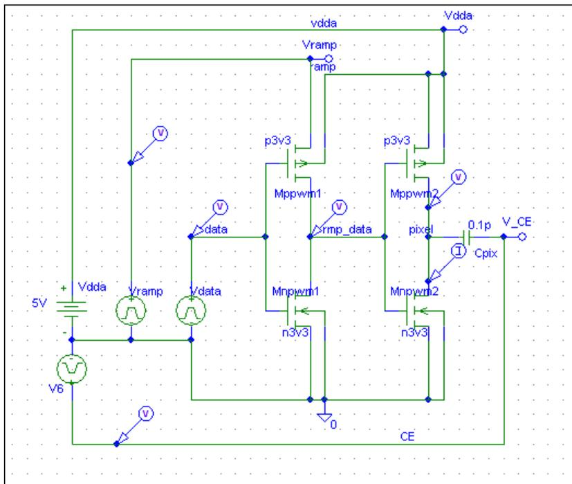
**Figure 5-15: a basic comparator circuit block for PWM**
