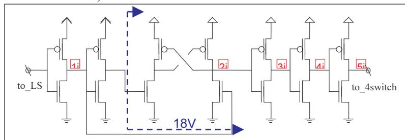
**Figure 6-59 : column driver level-shifter**
