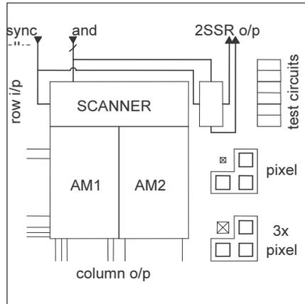
**Figure 6-2 : SiLCD chip floorplan**
