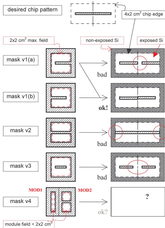
**Figure 3-4 : multiple-reticule and multiple-module approach**
