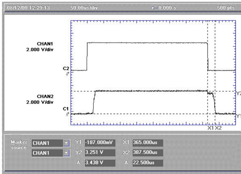
Figure 4-22: functional testing reveals a problem in the clock buffer tree
