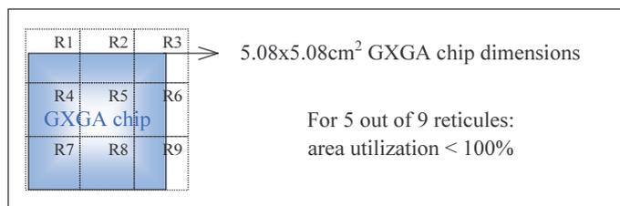
**Figure 3-2: many reticules per MOSAREL masking step**
