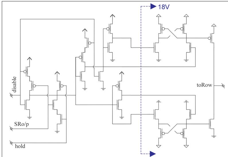
**Figure 6-63 : row driver logic and level shifter**
