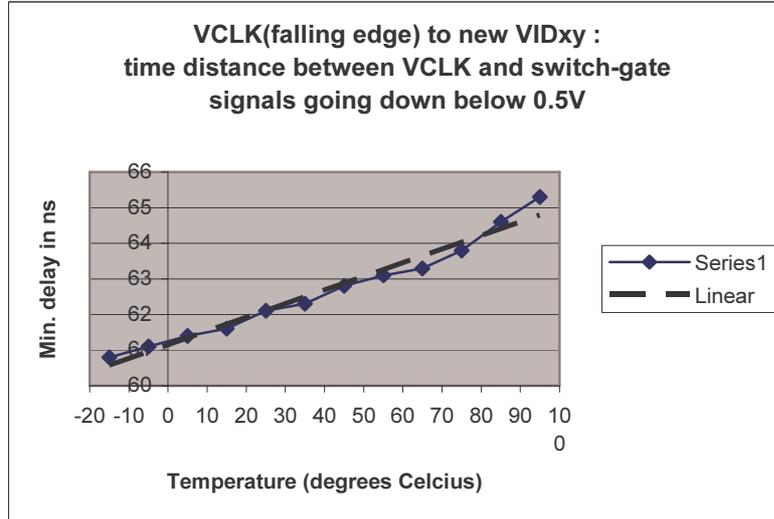
Figure 6-29 : temperature dependence of clock - video switch delay
