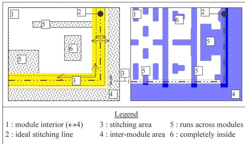
Figure 3-14 : anatomy of a module's layout
