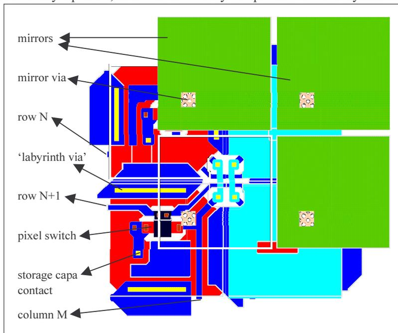
**Figure 4-11: 'reflec' pixel layout - layered view**
