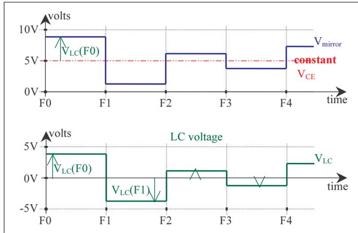
**Figure 5-2:  $V_{\text{mirror}}$  with respect to chip ground and resulting  $V_{\text{LC}}$**
