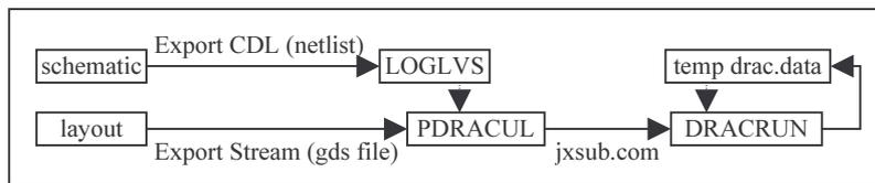
**Figure 7-85 : schematic operation of a dracula job**
