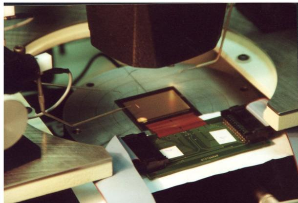
Figure 4-21: usage of probe-needles to measure inside the chip
