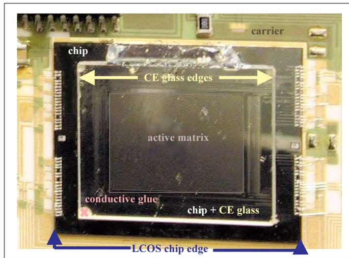
Figure 2-20 : 160x120 example of CE contact towards the chip
