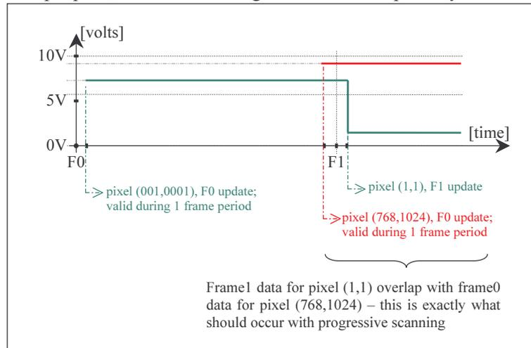
**Figure 4-8: frame updating mechanism**
