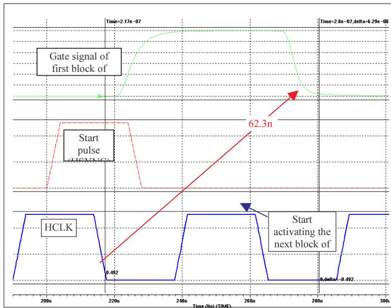
Figure 6-30 : video switch delay simulation at 25 C
