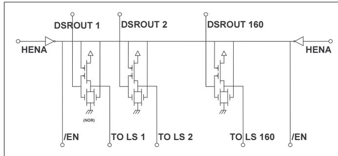
Figure 6-34 : enable circuit inside a column driver segment
