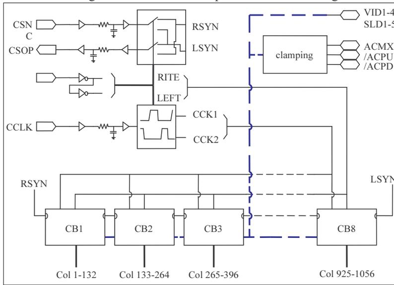
**Figure 6-54 : block schematic of the column driver**
