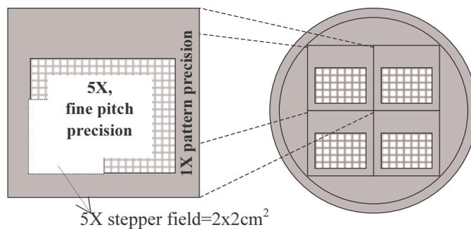
**Figure 3-3: the MOSAREL test-vehicle chip layout and the wafer layout. Coarse, non-repetitive features occur outside the fine-pitch display area**
