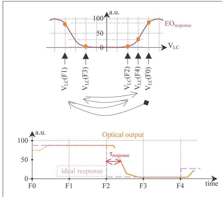
Figure 4-6: optical response to changes in  $V_{RMS}$
