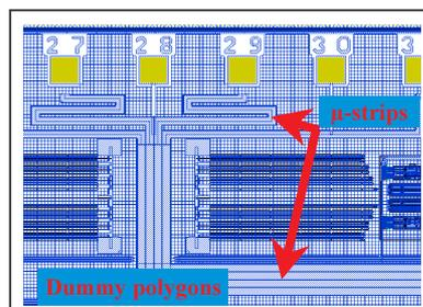
**Figure 2-15 : dummy polygons and de-coupling of signals with  $\mu$ -trips**
