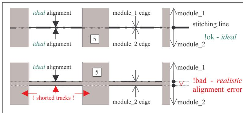
**Figure 3-15 : ideal bounding boxes vs. realistic alignment**
