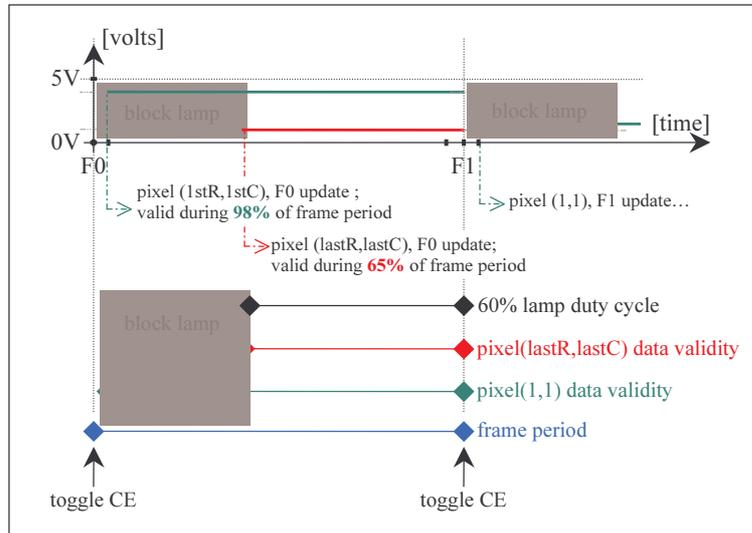
**Figure 5-5: 'concentrated' write cycles and light flow shutter**
