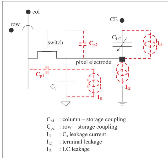
**Figure 4-3: parasitic components in the DRAM pixel**
