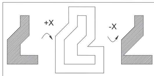
Figure 6-78 : +x, -x results in 'undergrow'; DRC min notch width should be  $> 2x$
