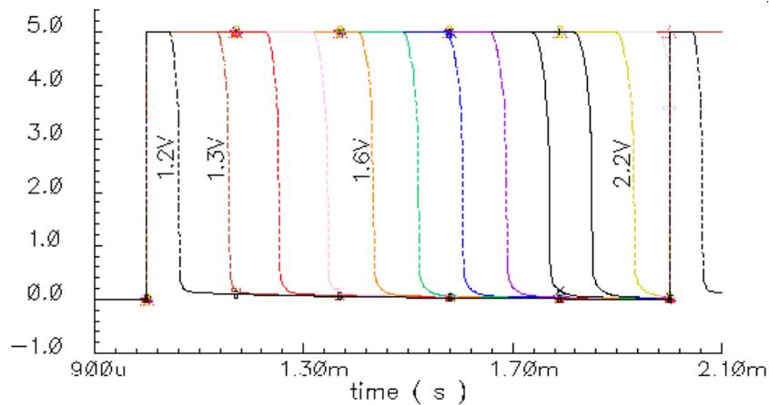
**Figure 5-16 : basic PWM circuit behavior (see figure 5-15)**
