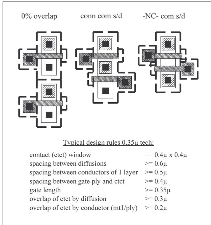
**Figure 5-6: impact of circuit configurations on layout area**
