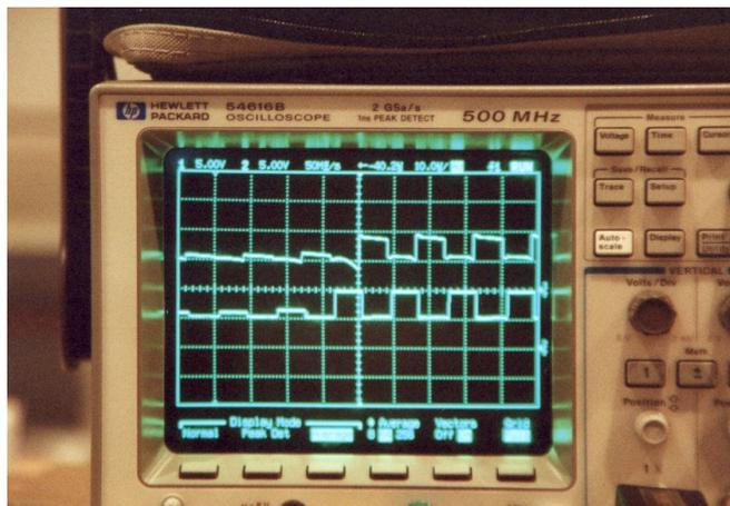
Figure 4-24: testing the same shift register,
