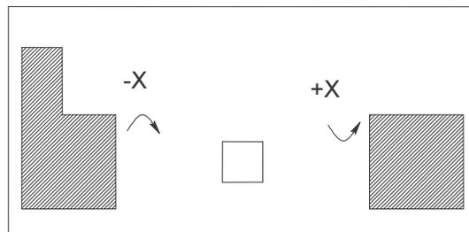
Figure 6-79 : -x,+x eliminates too thin (portions of) patterns, ok
