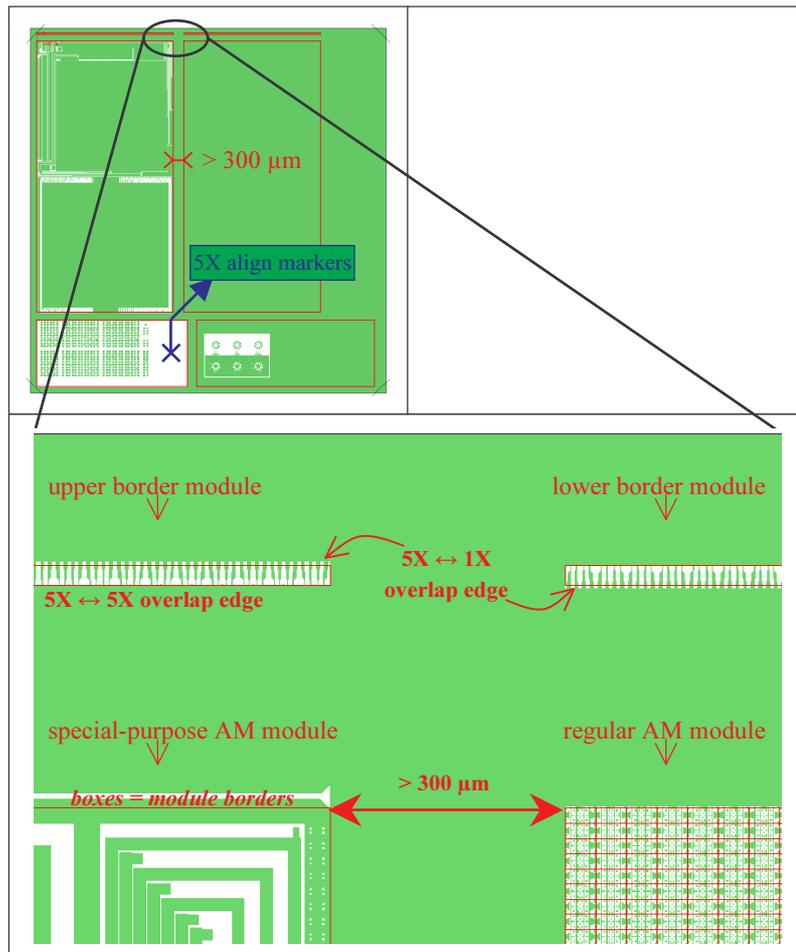
**Figure 2-27 : 5X mask drawing details**
