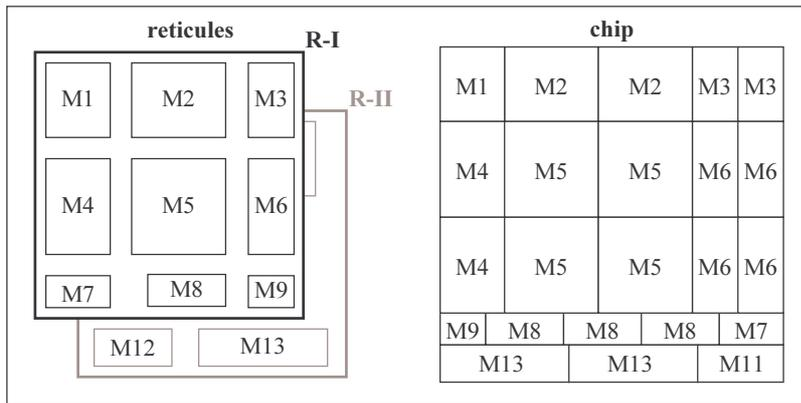
**Figure 3-7 : modular stitching principle**
