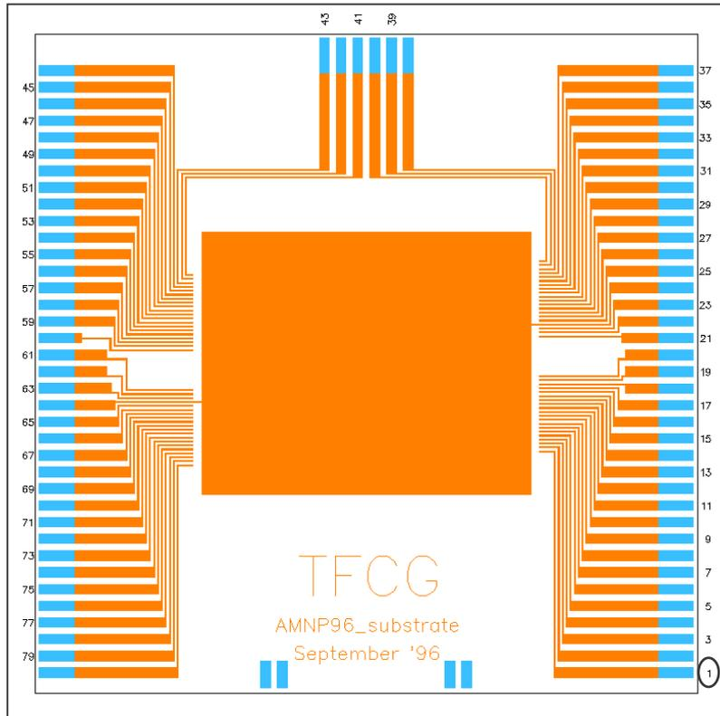
**Figure 6-9 : first version of the backplane carrier layout (5cm x 5cm)**
