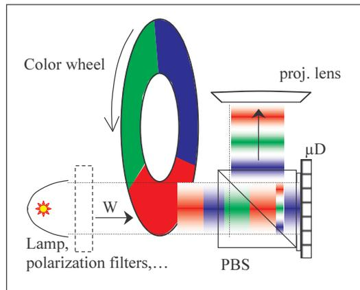
**Figure 1-8: single panel, frame sequential color architecture**
